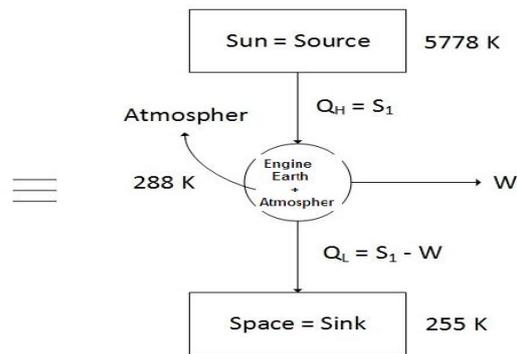
Figure 1. Control volume I (Sun (heat source), Earth and atmosphere (engine), space (heat sink)).
