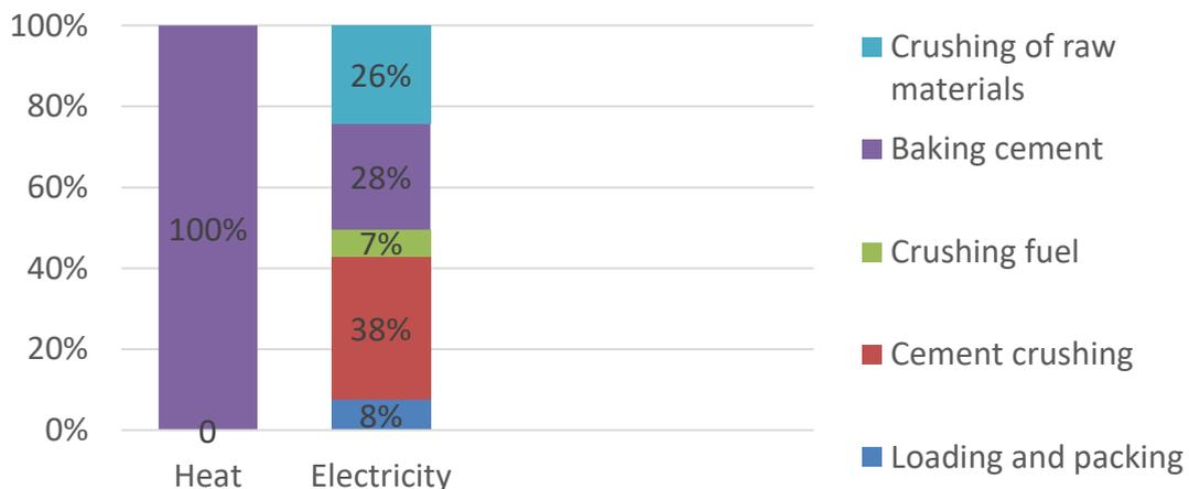
Figure 4. Type and scale of energy consumption in a cement production process [11].
