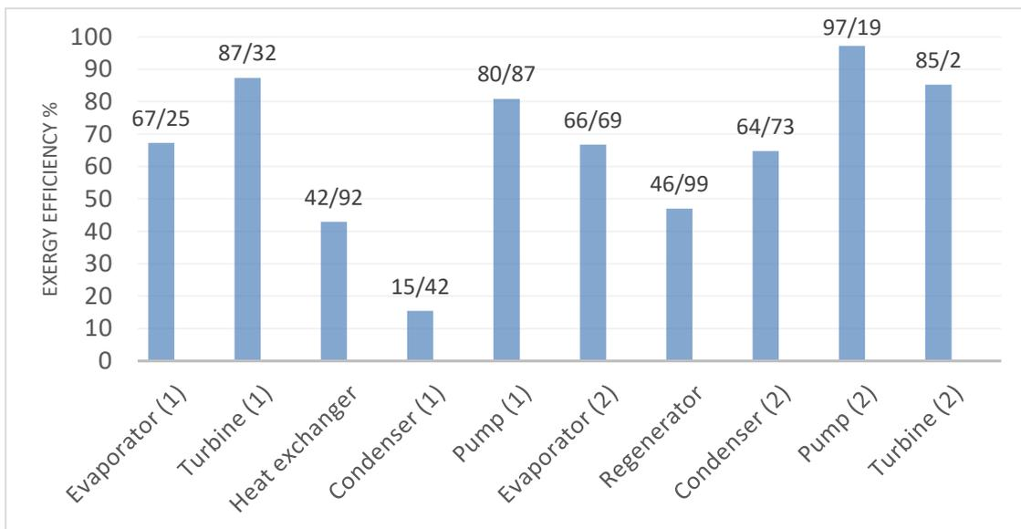
**Figure 7. Exergy efficiency of each component of system.**
