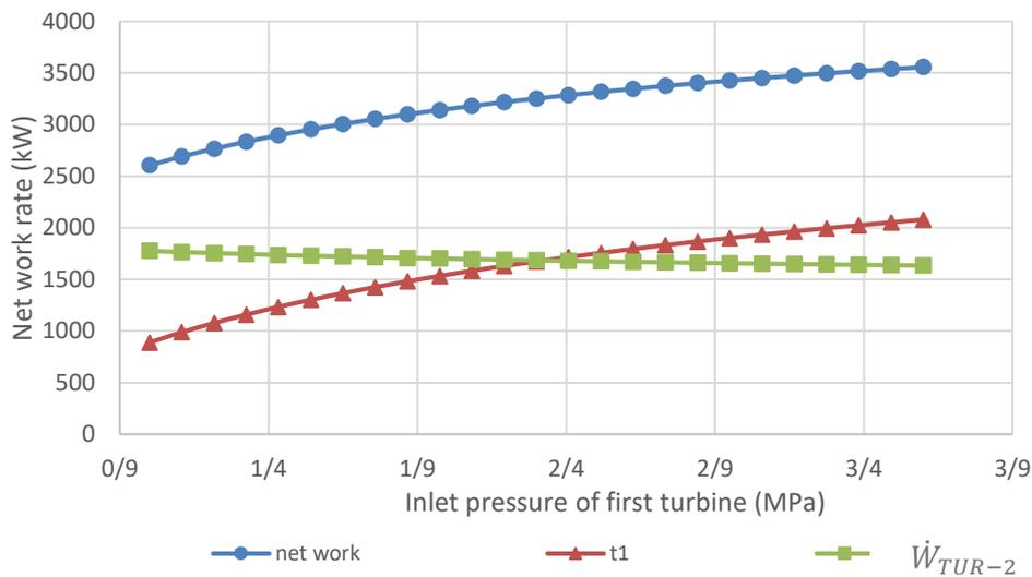
Figure 8. Influence of inlet pressure of first turbine on net work rate.
