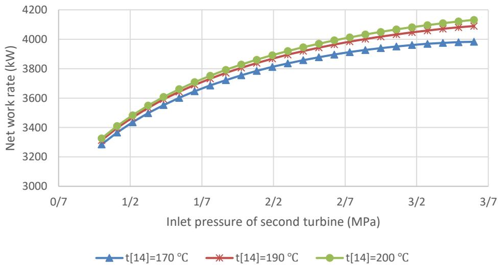
Figure 13. Influence of inlet pressure of second turbine on net work rate at different temperatures.
