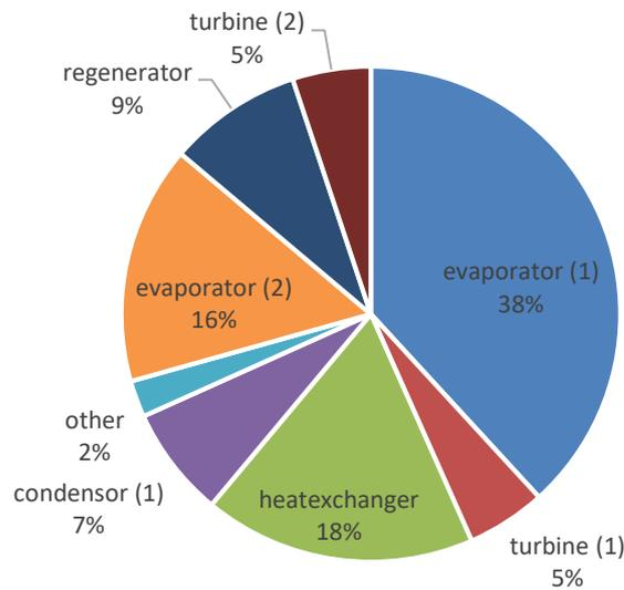
**Figure 6. Exergy destruction of each component of system.**
