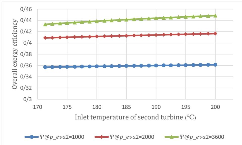
Figure 15. Influence of inlet temperature of second turbine on the exergy efficiency of the whole cycle.
