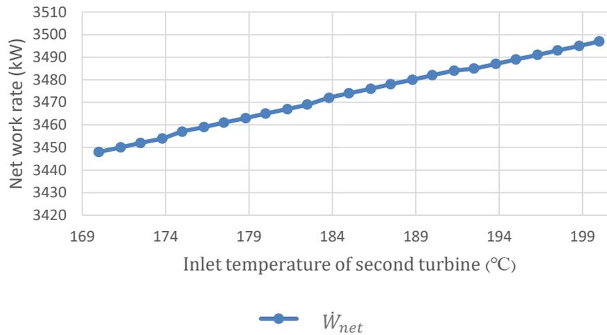
Figure 11. Influence of inlet temperature of second turbine on net work rate.
