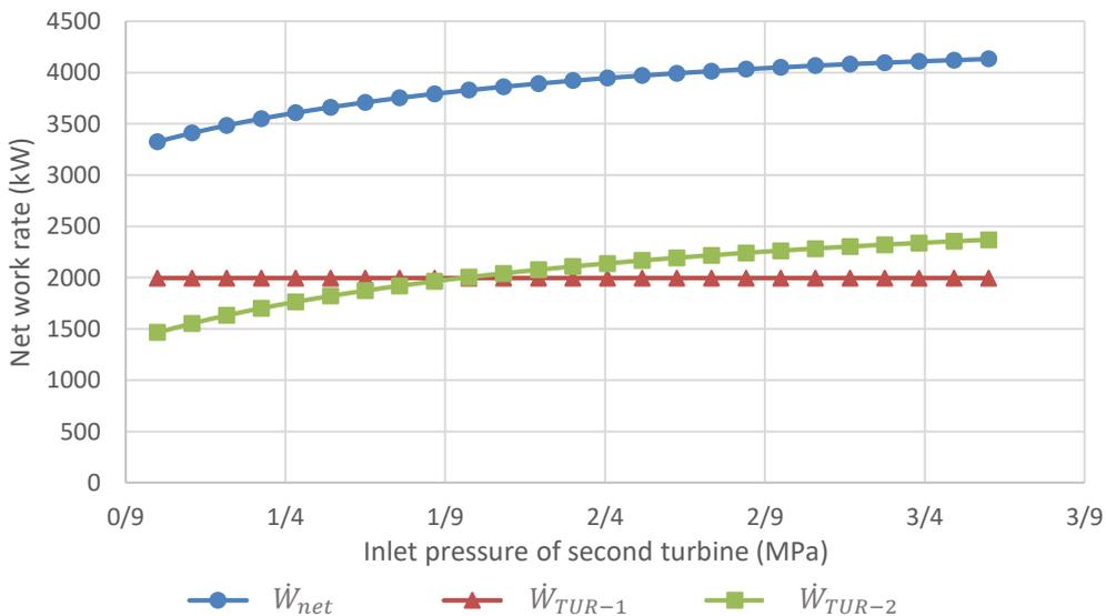
Figure 9. Influence of inlet pressure of second turbine on net work rate.
