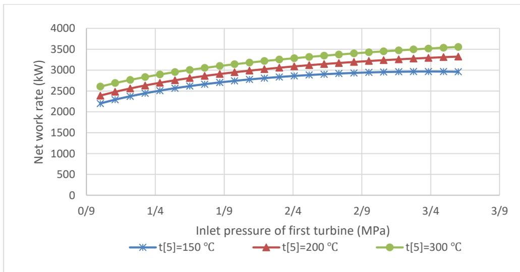
Figure 12. Influence of inlet pressure of first turbine on net work rate at different temperatures.
