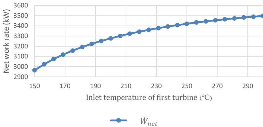
Figure 10. Influence of inlet temperature of first turbine on net work rate.
