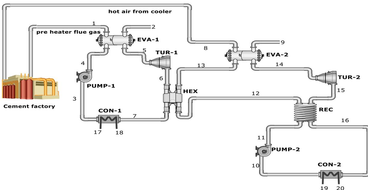
Figure 5. Schematic representation of the thermal recycling cycle.
