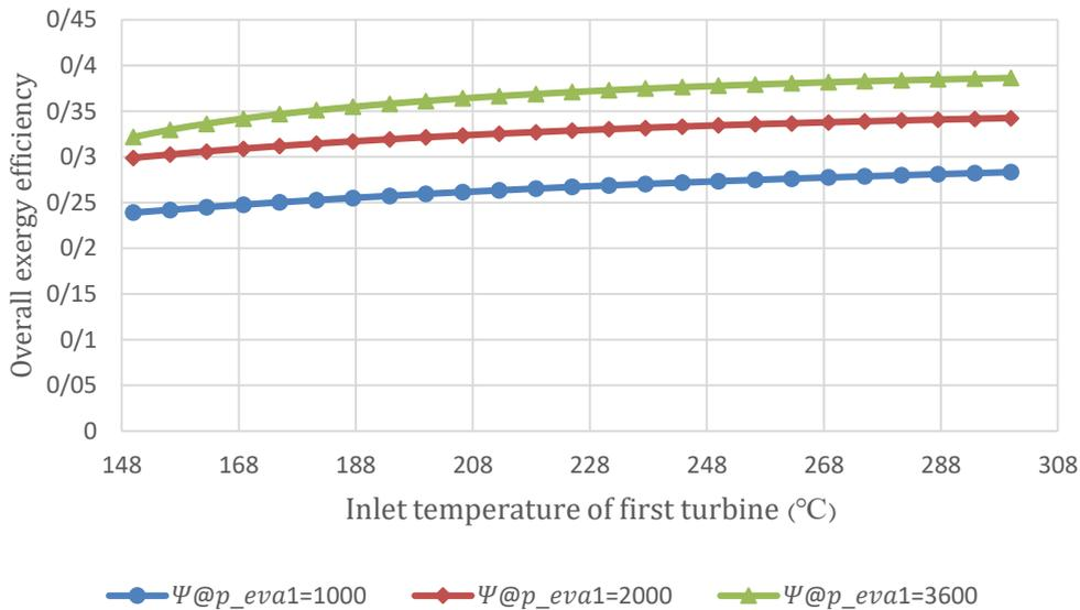
Figure 14. Influence of inlet temperature of first turbine on the exergy efficiency of the whole cycle.
