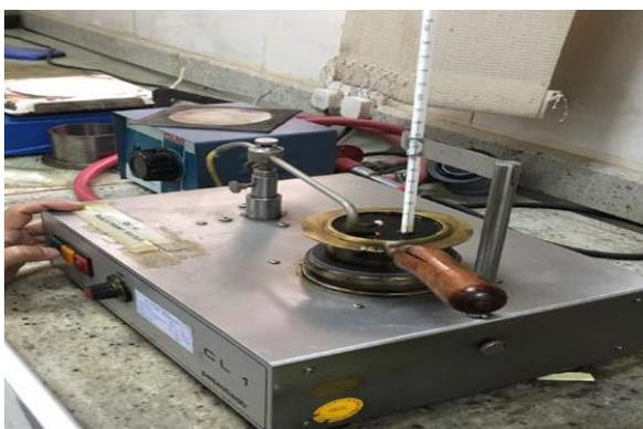
Figure 2. Flash point testing.
