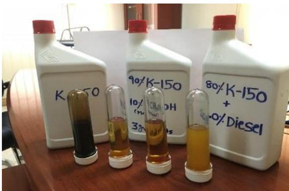
Figure 1. Samples of used engine oil and DLF after different treatment methods.
