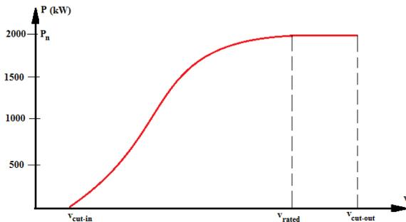
Figure 1. Non-linear wind power curve.
