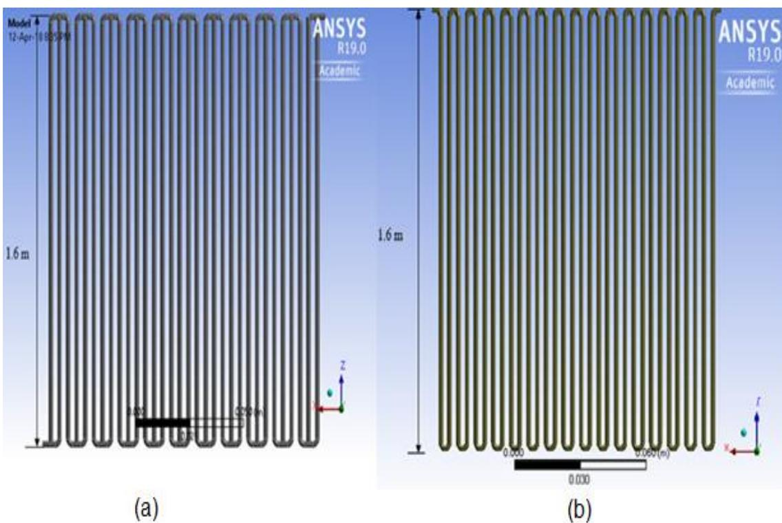
**Figure 2. Parallel series flow design. (b) Series flow design.**
