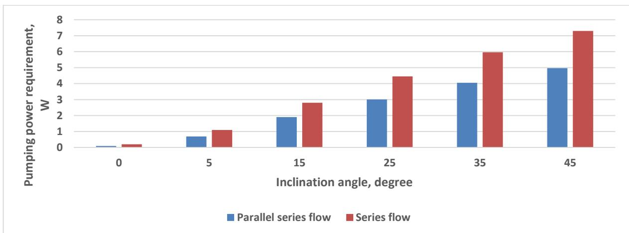
Figure 6. Effect of inclination angle on the pumping power requirement at a mass flow rate of 0.03 kg/s.
