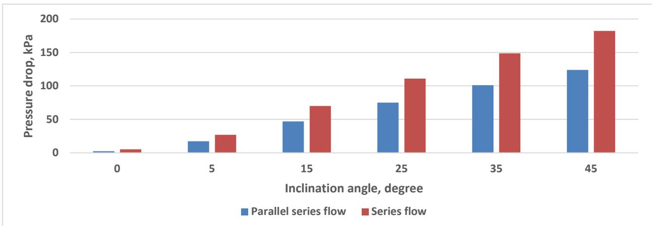
Figure 5. Effect of inclination angle on pressure drop at a mass flow rate of 0.03 kg/s.
