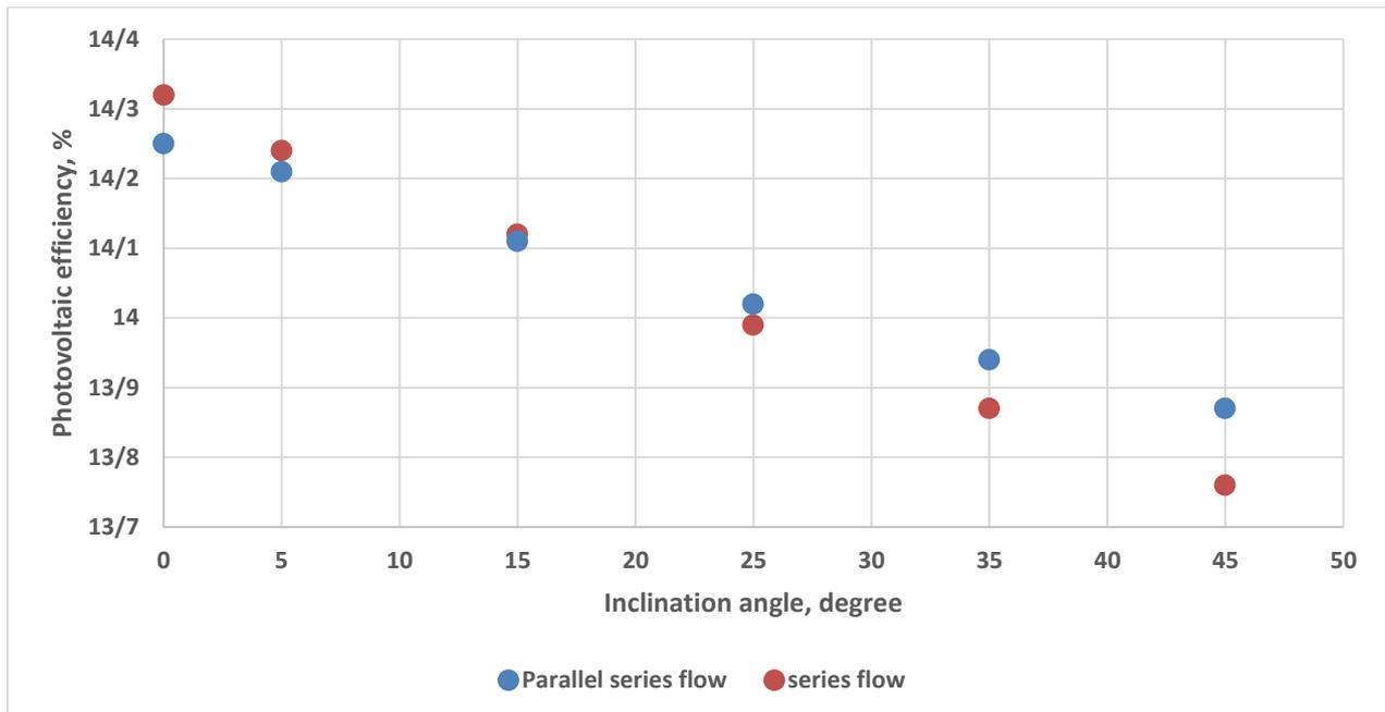
Figure 7. Effects of the inclination angle on the photovoltaic efficiency ( $I = 1000 \text{ W/m}^2$ ,  $\dot{m} = 0.03 \text{ kg/s}$ ,  $T_{in} = 25^\circ\text{C}$ ,  $T_a = 25^\circ\text{C}$ ).
