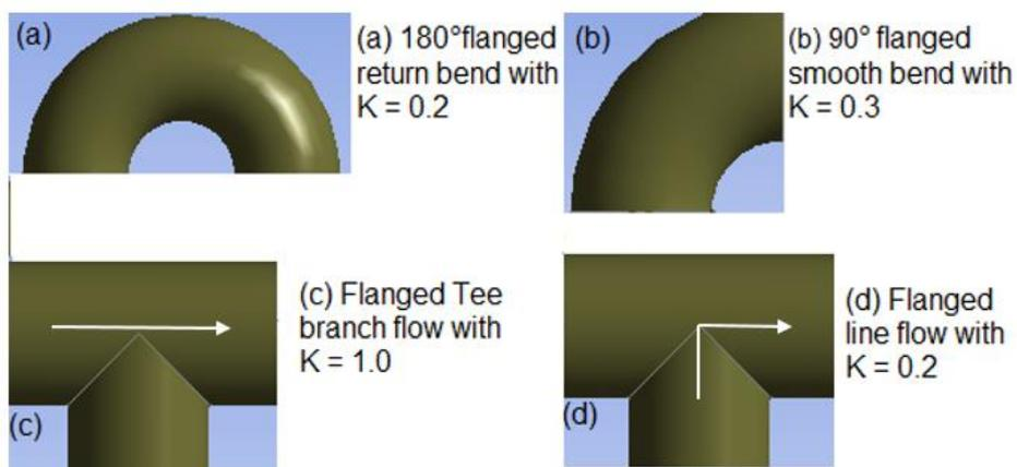
**Figure 3. Different pipe fittings with equivalent loss coefficients.**
