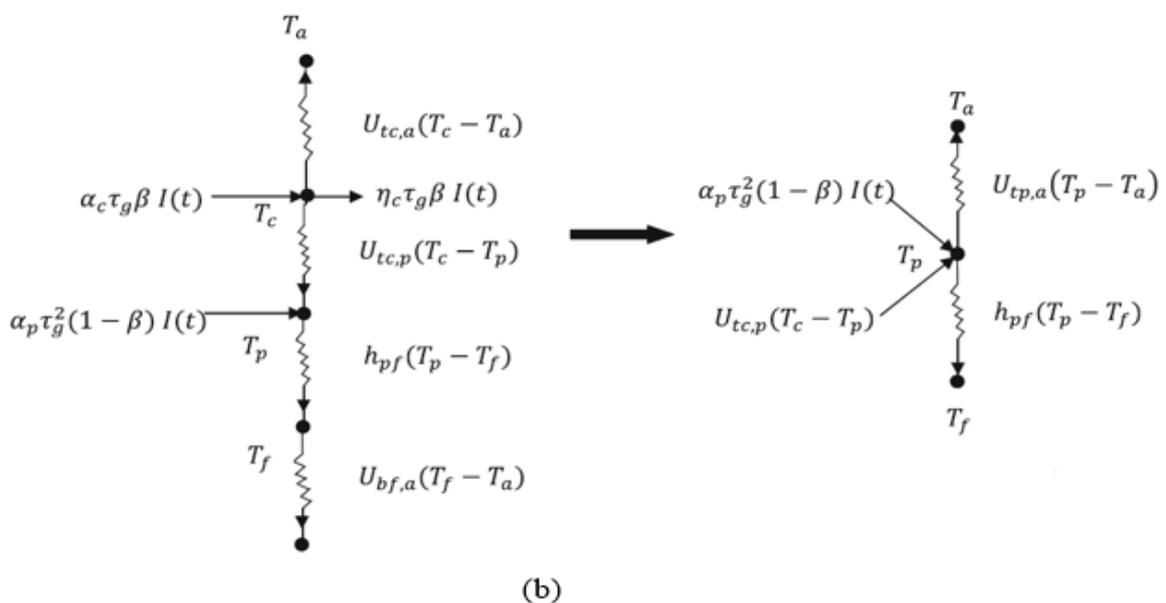
**Figure 4. (a) The different layers of the water based semi-transparent PVT. (b) The associated thermal network of the semi-transparent PVT [39]**
