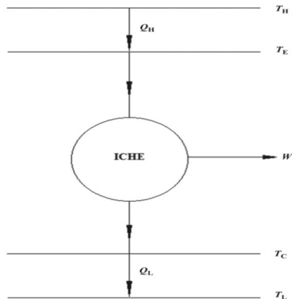
Figure 1. Diagram of irreversible Carnot heat engine (ICHE).
