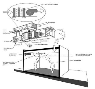
Figure 5. How UVC can be utilized to reduce pathogens in indoor air and on surfaces, while being installed in-duct and upper-room level. Source: [16].
