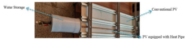
Figure 3. Photo of conventional PV and PV equipped with heat pipe and their layout on system.
