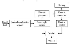
Figure 3. Structure of a compound hybrid electric vehicle.
