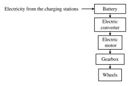
Figure 7. Structure of an all-electric vehicle.
