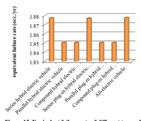
Figure 15. Equivalent failure rate of different types of electric vehicles.
