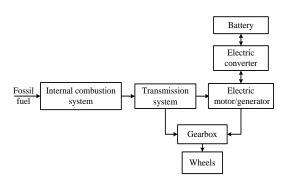
Figure 2. Structure of a parallel hybrid electric vehicle.
