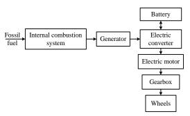
Figure 1. Structure of a series hybrid electric vehicle.
