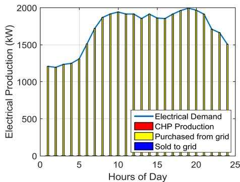
Figure 13. Electrical demand and production capacities for  $P_{CHP} = 0$  kW when type II CHP is used.
