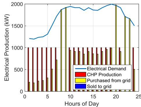
Figure 15. Electrical demand and production capacities for  $P_{CHP} = 1000$  kW when type II CHP is used.
