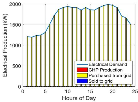
Figure 5. Electrical demand and production capacities for  $P_{CHP} = 0 \text{ kW}$  when type I CHP is used.
