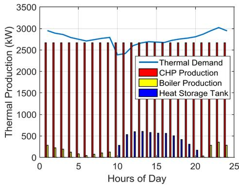
Figure 18. Thermal demand and production capacities for  $P_{CHP} = 2000 \text{ kW}$  when type I CHP is used.
