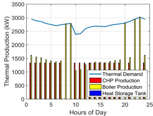
Figure 16. Thermal demand and production capacities for  $P_{CHP} = 1000$  kW when type II CHP is used.
