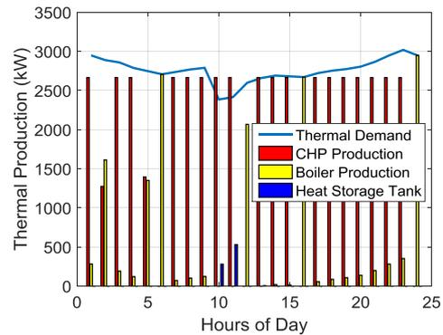
Figure 10. Thermal demand and production capacities for  $P_{CHP} = 2000 \text{ kW}$  when type I CHP is used
