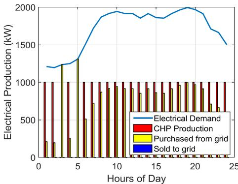
Figure 7. Electrical demand and production capacities for  $P_{CHP} = 1000 \text{ kW}$  when type I CHP is used.
