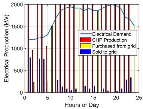
Figure 9. Electrical demand and production capacities for  $P_{CHP} = 2000 \text{ kW}$  when type I CHP is used.
