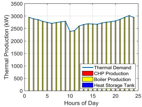
Figure 14. Thermal demand and production capacities for  $P_{CHP} = 0$  kW when type II CHP is used.
