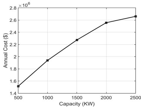
Figure 12. Annual cost of CHP in terms of its production capacity when type II CHP is used.
