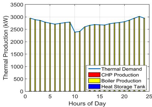
Figure 6. Thermal demand and production capacities for  $P_{CHP} = 0 \text{ kW}$  when type I CHP is used.
