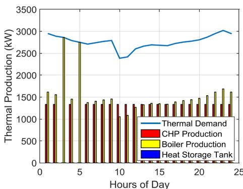
Figure 8. Thermal demand and production capacities for  $P_{CHP} = 1000 \text{ kW}$  when type I CHP is used.
