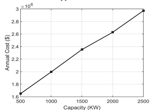
**Figure 4. Annual cost of CHP in terms of its production capacity when type I CHP is used.**
