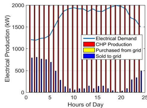
Figure 17. Electrical demand and production capacities for  $P_{CHP} = 2000$  kW when type II CHP is used.
