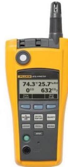
Figure 1. Fluke 975 air-meter.
