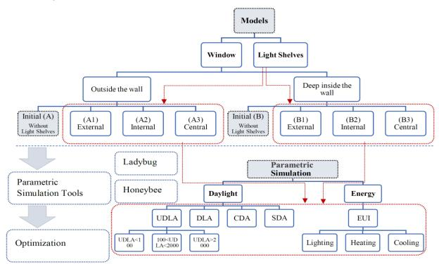
Figure 1. Research framework: daylight and energy optimization process and tools.
