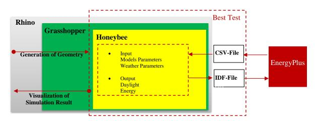
Figure 2. Data processing in Honeybee; validation performance can be identified at the blue dashed line border.
