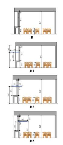
Figure 4. Different placement models for installing light shelves in the study.
