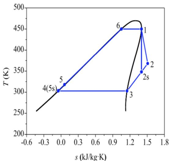
Figure 1. T-s diagram of an ORC [24].
