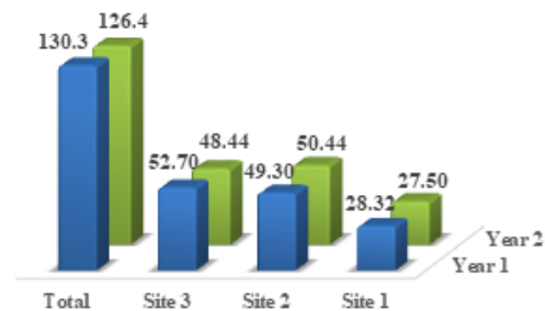
Figure 4. Reduction of NG consumption due to the energy yields by the studied wind farms (million m 3 ).
