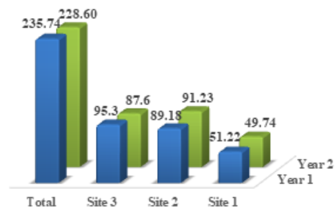
Figure 6. CO 2 reductions due to the energy yields of the studied wind farms regarding the considered gas-cycle power plant and NG fuel intake (thousand tons).
