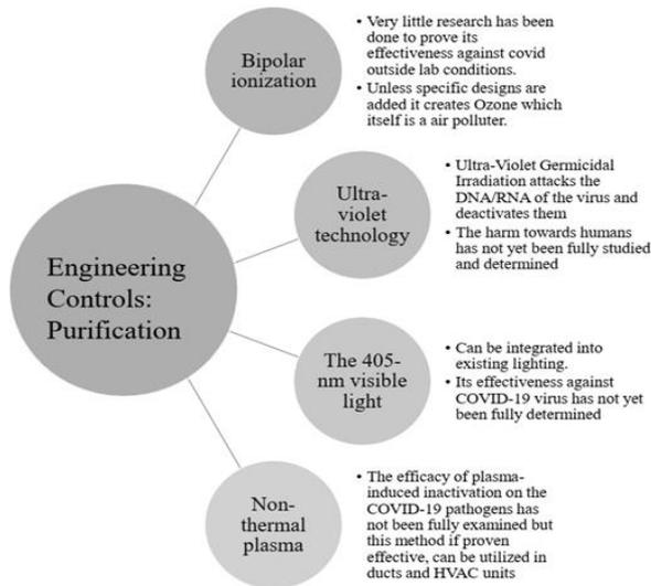
Figure 3. Engineering control measures in regard to purification.
