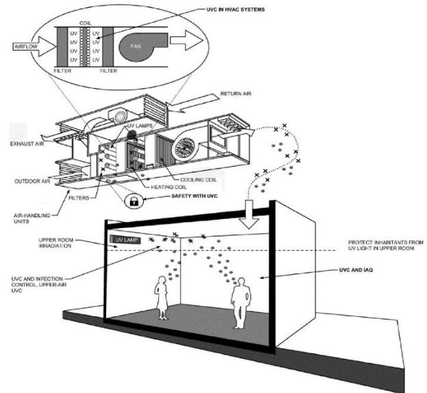
Figure 5. How UVC can be utilized to reduce pathogens in indoor air and on surfaces, while being installed in-duct and upper-room level. Source: [16].
