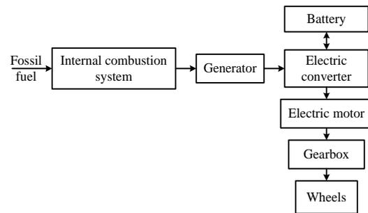
**Figure 1. Structure of a series hybrid electric vehicle.**
