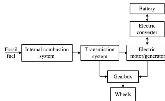
**Figure 2. Structure of a parallel hybrid electric vehicle.**
