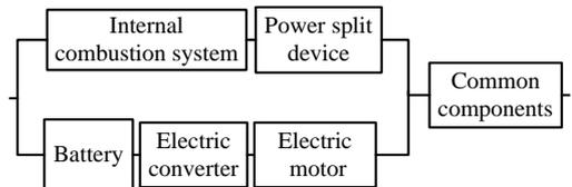
Figure 13. Reliability model of compound hybrid electric vehicle.
