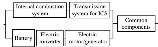
Figure 12. Reliability model of parallel hybrid electric vehicle.
