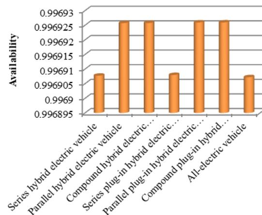
**Figure 16. Availability of different types of electric vehicles.**
