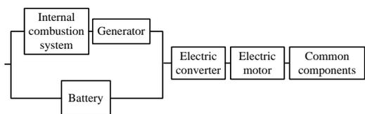
Figure 9. Reliability model of series hybrid electric vehicle.
