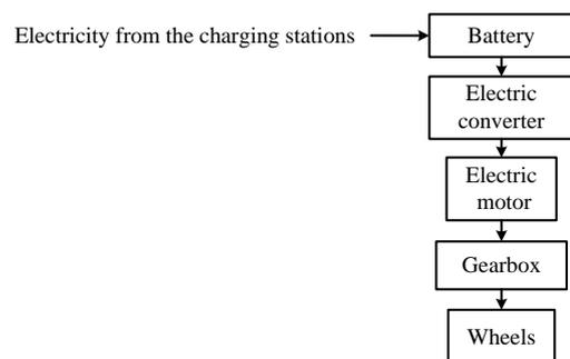
Figure 7. Structure of an all-electric vehicle.
