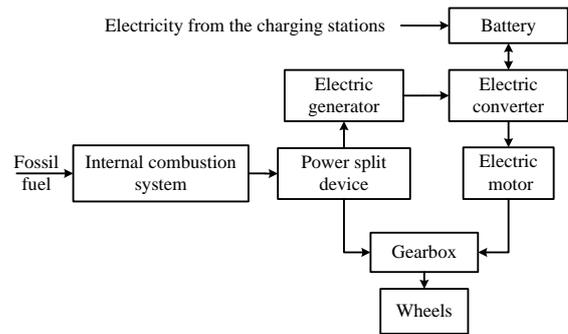
Figure 6. Structure of a compound plug-in hybrid electric vehicle.
