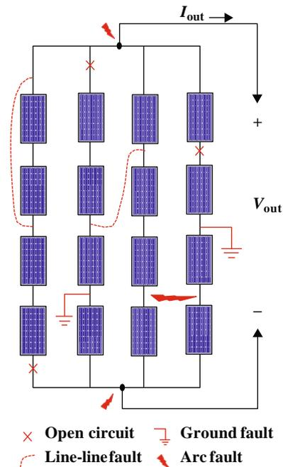
Figure 2. Most usual faults occur in PVs based on their location.
