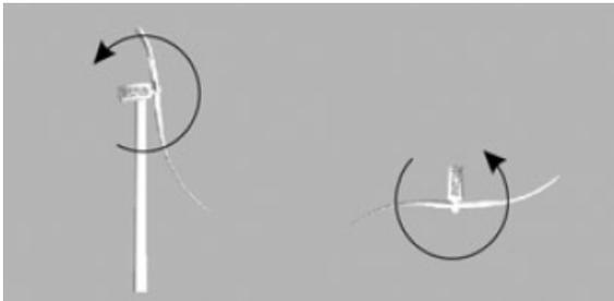
Figure 17. Schematic description of asymmetric out of plane bending mode of rotor 0.
