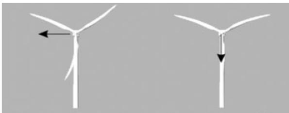
**Figure 7. Schematic description of asymmetric edge-wise bending mode of rotor 0.**
