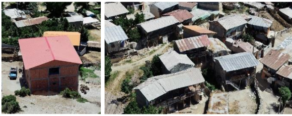
Figure 4. A representation of the dense point cloud used to generate DSM.
