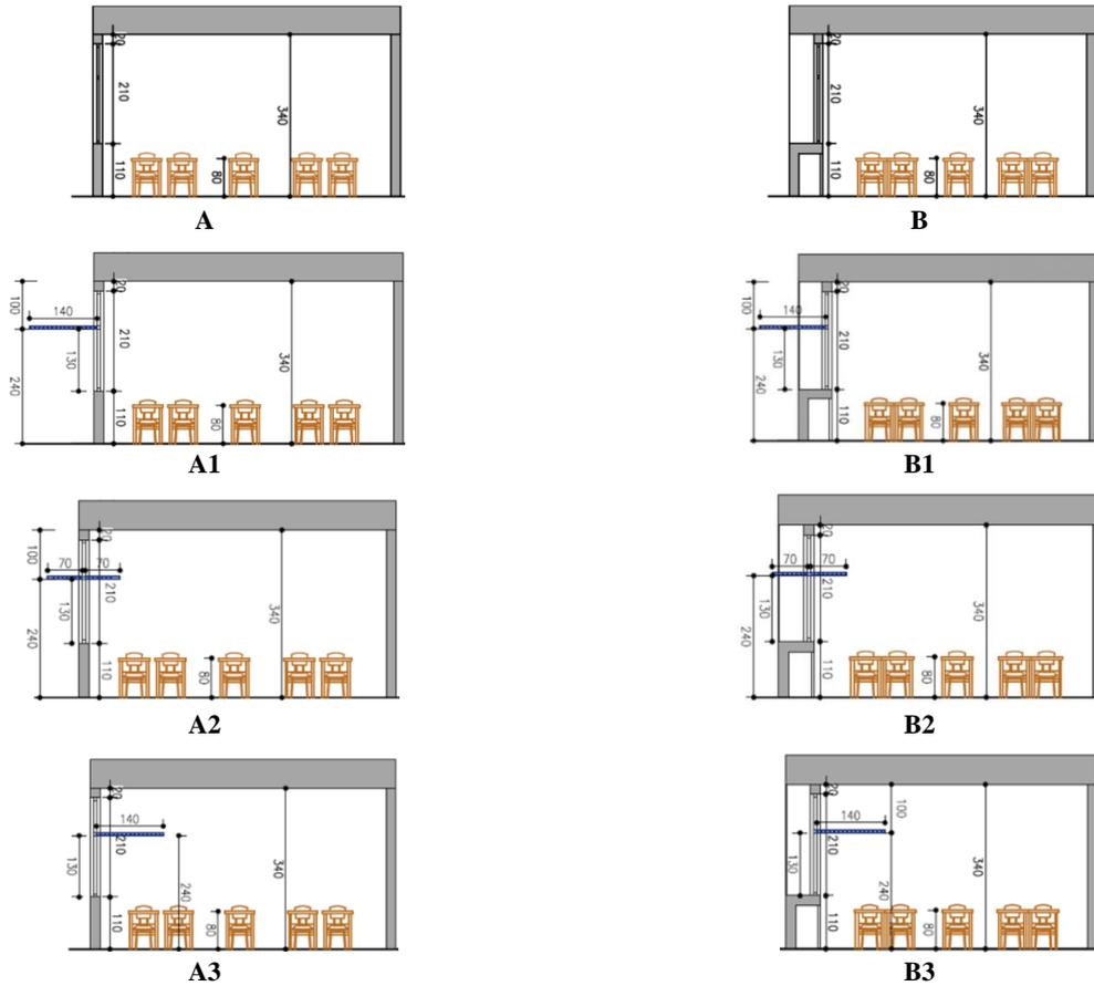
Figure 4. Different placement models for installing light shelves in the study.
