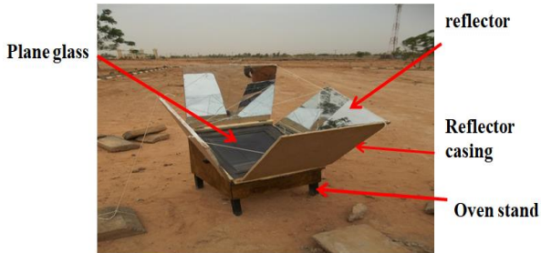
Figure 9. Four-reflector solar baking oven
