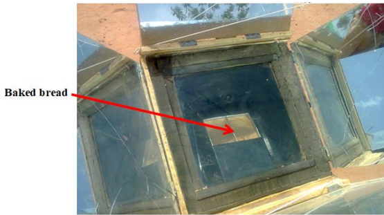
Figure 10. Experimental setup of the solar oven.
