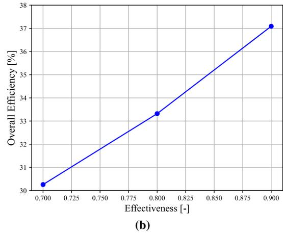
Figure 2. Effect of heat exchanger effectiveness on a) mass flow rates of the streams and b) overall efficiency.
